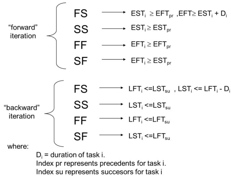
Figure 1: Calculations for the EST, EFT, LST and LFT using the proposed algorithm.
