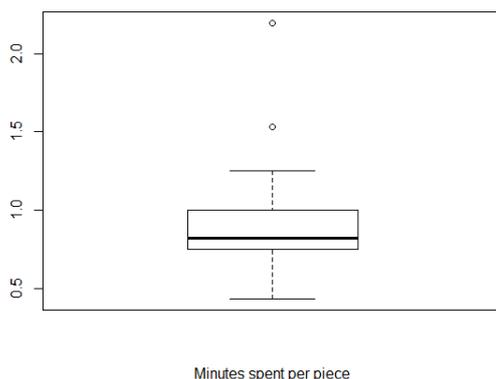
Figure 3. Number of minutes spent per piece on the saw cutting subprocess.
