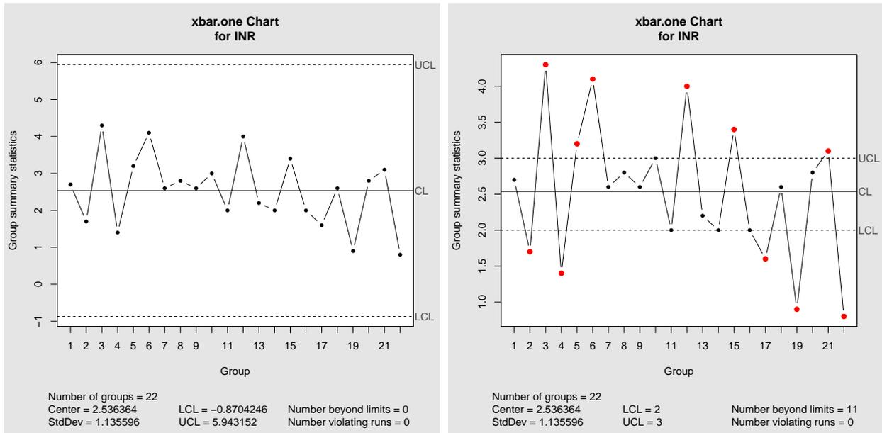
(a) Shewhart control chart with 3 $\sigma$  control limits. (b) Shewhart control chart with INR acceptable limits.
