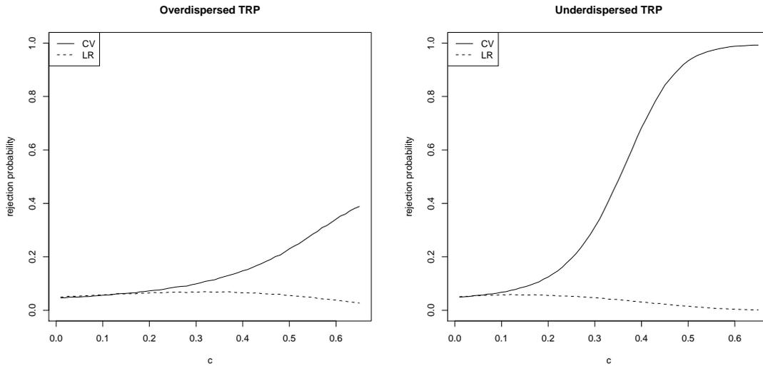
Figure 4: Simulations of TRPs with underlying Weibull RPs with shape parameter  $\beta = 0.75$  (overdispersed) and  $\beta = 1.5$  (underdispersed TRP), trend function displayed in Figure 3 and expected number of failures in each phase equal to 20.
